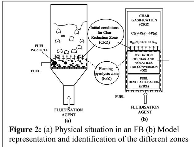
Figure 2: (a) Physical situation in an FB (b) Model representation and identification of the different zones
