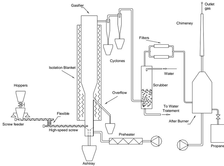
**Figure 1.** BFB 150 kW<sub>th</sub> pilot plant facility
